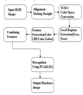
Fig.5. System block diagram of color FR framework based on color local texture features
