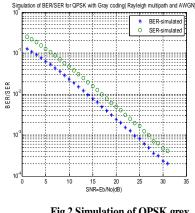
Fig 2 Simulation of QPSK grey coding
