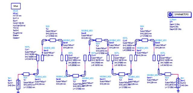
Fig. 1. Schematic view of hairpin filter
