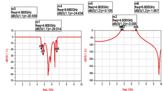
Fig.8. Simulated performance of combline filter in FR4
