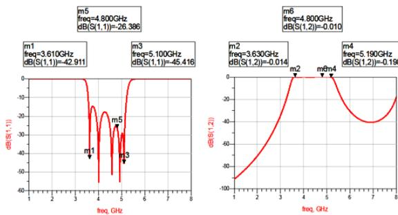
Fig.4. Simulated performance of hairpin filter in RT/Duroid 6010
