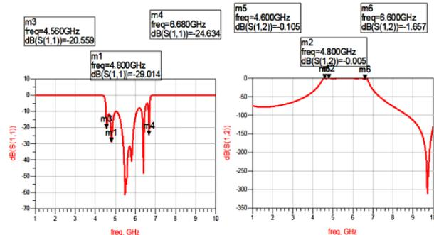
Fig.10. Simulated performance of combline filter in RO3010
