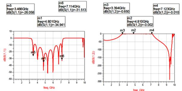
Fig.9. Simulated performance of combline filter in RT/Duroid 6010
