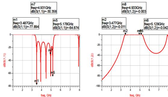
Fig.5. Simulated performance of hairpin filter in RO3010
