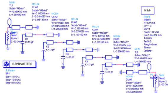
Fig.6. Schematic view of combline filter
