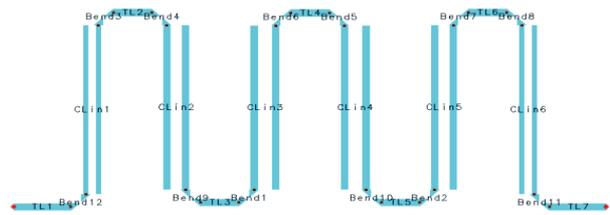
Fig. 2. Layout view of hairpin filter
