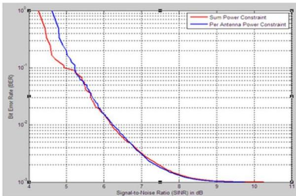
Fig.4. Plot of SINR in dB vs. BER
