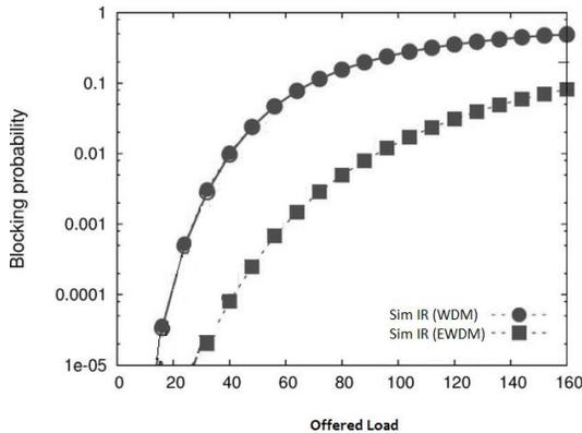
Fig. 5 Load versus Blocking Probability.
