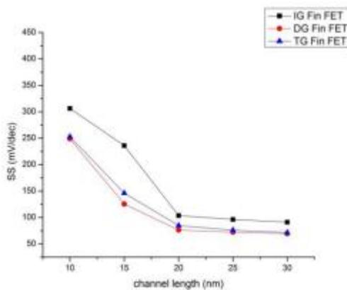
Fig-3(d) Subthreshold Swing (SS) over different channel lengths of 3D FinFETs
