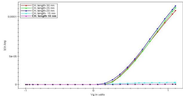
Fig-3(a) Drain current(I<sub>d</sub>) Vs Gate voltage (V<sub>g</sub>) of SiO<sub>2</sub> gate oxide DG FinFET varying channel length.
