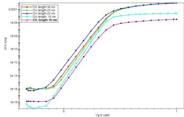
Fig-3(b) logarithmic drain current variation of Figure-3(a)
