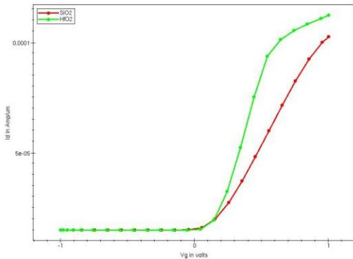
Fig-2 Drain current(I<sub>d</sub>) Vs Gate voltage (V<sub>g</sub>) of FinFET using different gate oxide
