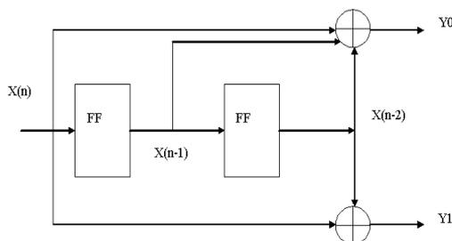
Fig. 6 Convolutional encoder
