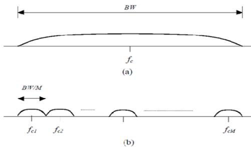
Fig 4 a) PSD of wide band single carrier direct sequence
