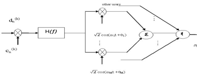
Fig 5 Block Diagram Of Multi Carrier Direct Sequence CDMA
