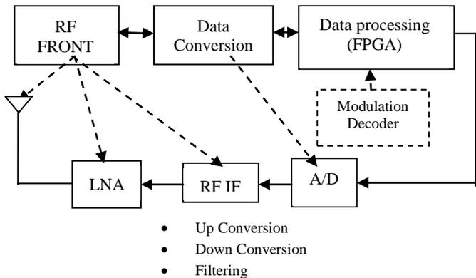
Fig 1 : SDR system Architecture
