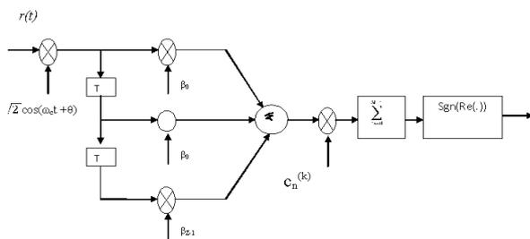
Fig. 7 Receiver System For Single Carrier
