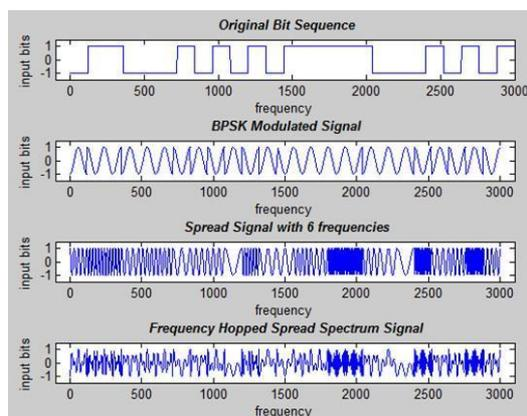
Figure 2 Inputs and Modulation of bitstreams
