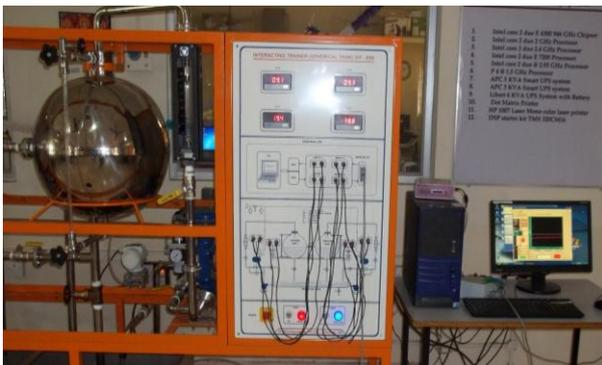
Fig. 2. Experimental set up for single spherical tank system.
