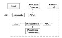
Fig.1. Block diagram of peak current mode control of buck- boost converter
