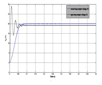
Fig.7. Comparison between open loop and closed loop output voltage waveforms
