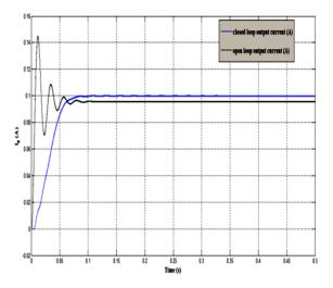
Fig.6. Comparison between open loop and closed loop output current waveforms
