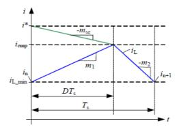
Fig.3. Inductor current characteristics to illustrate principle of digital slope compensation
