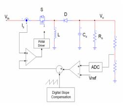
Fig.2. Digital peak current mode control of buck-boost converter
