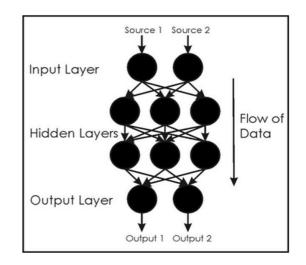
Fig.2.Architecture of simple Neural Network
