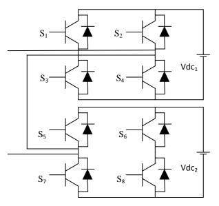
Fig. 1 CMLI with Separate DC Source
