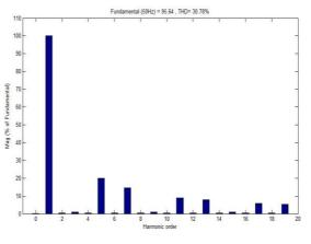
Fig. 7 Harmonic spectrum of Five level CMLI using GA
