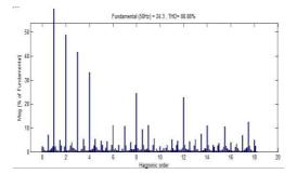
Fig. 5 Harmonic spectrum of Five level CMLI using N -R method.
