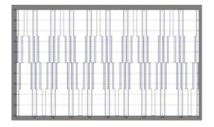
Fig. 4 Output waveform of five level CMLT using SHE Technique
