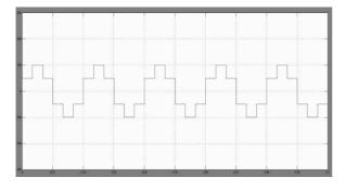
Fig. 6 Output waveform of Five Level Inverter
