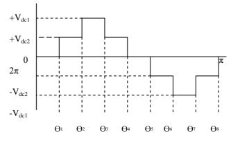
Fig. 2 The Synthesized Phase Voltage Waveform of Five level Cascaded Inverter.
