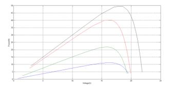
Fig.5 P-V characteristics of 50w Solar Panel
