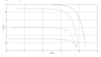
Fig.4 I-V characteristics of 50w Solar Panel
