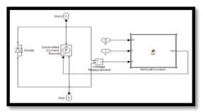
Fig.3 PV Model of Mat-lab-Simulink
