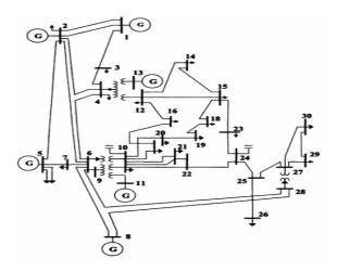
Fig.2. Single Line Diagram of IEEE-30 bus system
