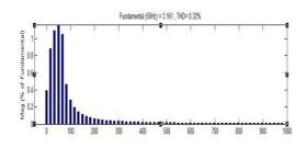
Fig. 15. FFT plot for current injected to the grid
