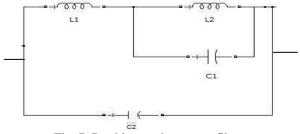
Fig. 7 Double tuned resonant filter
