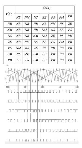
Fig. 8 CPWM scheme for switching of CSI
