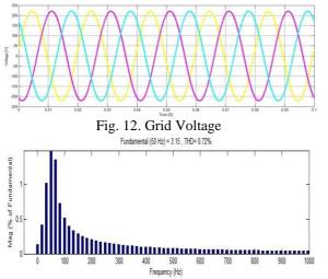
Fig. 13 FFT plot for voltage injected to the grid
