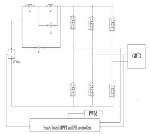
Fig. 3 Three phase grid connected current source inverter
