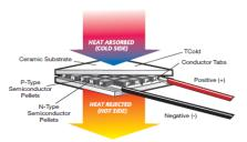
Fig.2 Complete Thermoelectric Module
