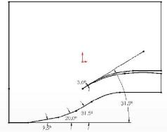
Figure 4 Geometry of Inlet
