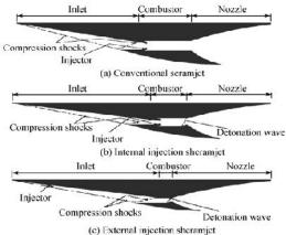
Figure 1 Hypersonic airbreathing vehicle scheme SCRAM JET ENGINE
