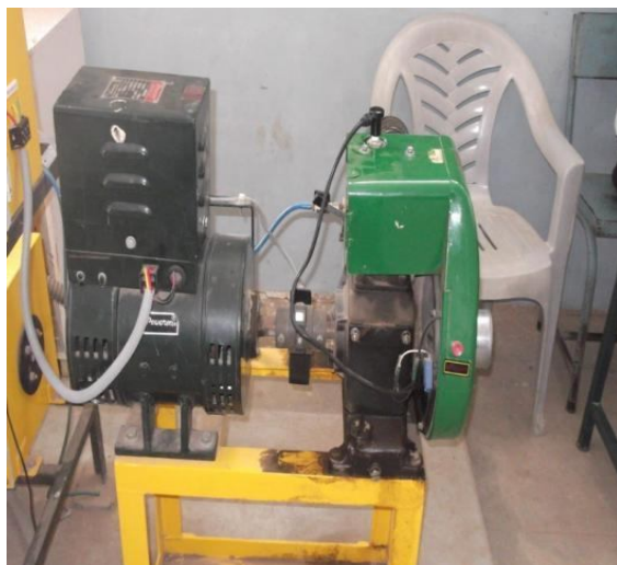
Fig 8 Four Stroke Engine With Electrical Generator
