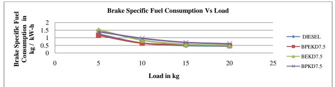
Fig: 8Comparasion of Break Specific Fuel Consumption for BPEKD7.5, BEKD7.5, BPKD7.5 and Pure Diesel
