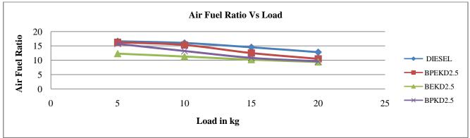
Fig: 10Comparasion of Air Fuel Ratio for BPEKD2.5, BEKD2.5, BPKD2.5 and Pure Diesel
