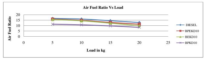
Fig: 13Comparasion of Air Fuel Ratio for BPEKD10, BEKD10, BPKD10 and Pure Diesel
