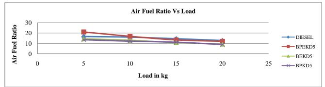
Fig: 11Comparasion of Air Fuel Ratio for BPEKD5, BEKD5, BPKD5 and Pure Diesel
