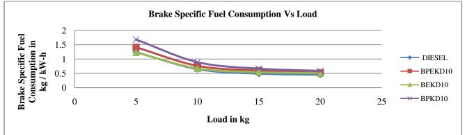
Fig : 9Comparasion of Break Specific Fuel Consumption for BPEKD10, BEKD10, BPKD10 and Pure Diesel
