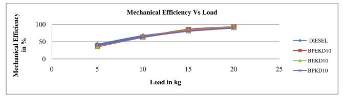
Fig : 5Comparasion of Mechanical Efficiency for BPEKD10, BEKD10, BPKD10 and Pure Diesel
