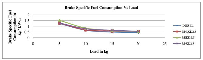
Fig: 6 Comparasion of Break Specific Fuel Consumption for BPEKD2.5, BEKD2.5, BPKD2.5 and Pure Diesel
