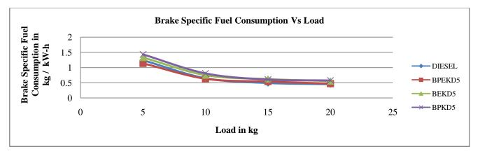
Fig: 7 Comparasion of Break Specific Fuel Consumption for BPEKD5, BEKD5, BPKD5 and Pure Diesel
