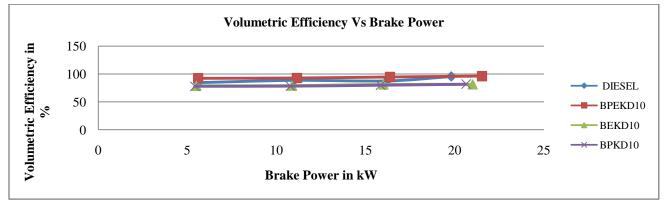
Fig: 14Comparasion of Volumetric Efficiency for BPEKD10, BEKD10, BPKD10 and Pure Diesel
