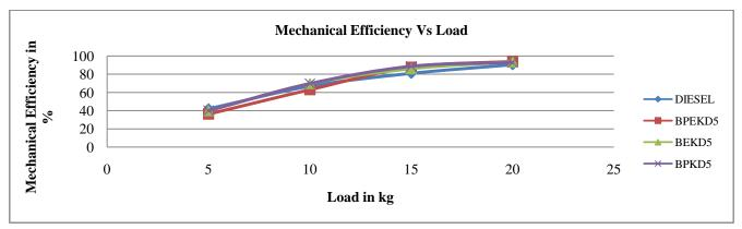
Fig : 3Comparasion of Mechanical Efficiency for BPEKD5, BEKD5, BPKD5 and Pure Diesel
