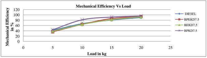
Fig: 4Comparasion of Mechanical Efficiency for BPEKD7.5, BEKD7.5, BPKD7.5 and Pure Diesel
