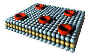
Figure1. Artificial ion channels (red cylinders) built into a threelayer nanomembrane.( Zoran Jaksic 2011)
