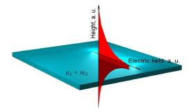
**Figure2.** Long-range surface-plasmon-polariton (SPP) propagation on a self-supported nanomembrane. "1; "2: Dielectric functions. a.u.: Arbitrary units.( Zoran Jaksic 2011)
