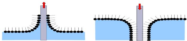
Figure 5. Schematic presentation of Langmuir-Blodget Technique for hydrophilic and hydrophobic substrates. (Zoran Jaksic 2010)
