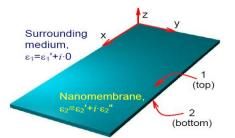
Figure 4. Basic configuration of a freestanding nanomembrane guide for long-range surface plasmon polariton propagation (metaldielectric interface) (Kenichi Takahata, 2009)
