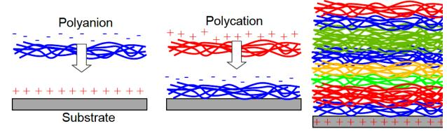
Figure 6. Layer-by-layer nanomembrane assembly technique. Left: assembly of the first layer; middle: assembly of the second layer; right: final structure (.Zoran Jaksic 2010)
