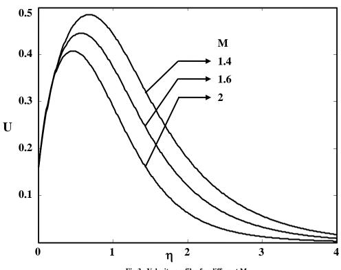
Fig.3 Velocity profiles for different M
