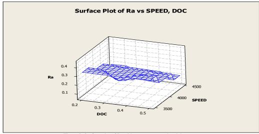
Figure 3: Surface plot of R<sub>a</sub> with respect to speed and doc
