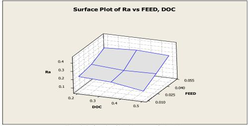
Figure 2: Surface plot of Ra with respect to feed and doc
