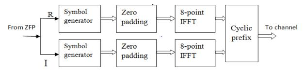
Fig 4 OFDM modulator block diagram.
