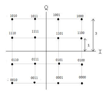
Fig 3 QAM-16 Constellation diagram
