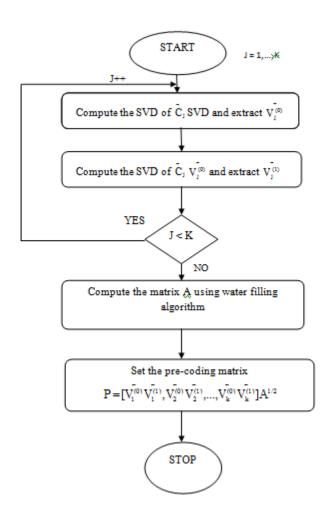
Fig 1. Flow chart of zero-forcing algorithm.
