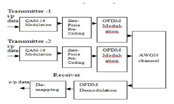
Fig 2 Block diagram of Zero-force pre-coded MIMO channel
