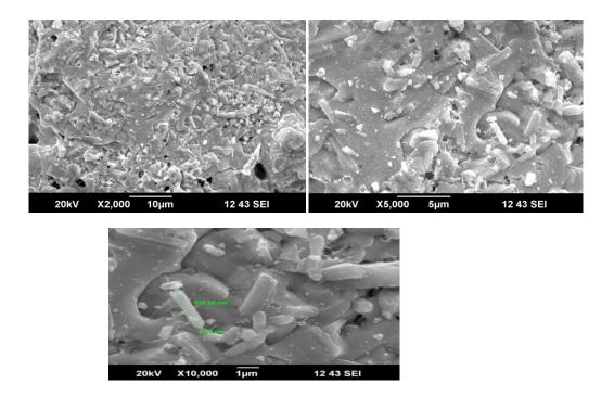
Fig.4. SEM images of BaBiO<sub>3</sub> pervoskite at different magnificence
