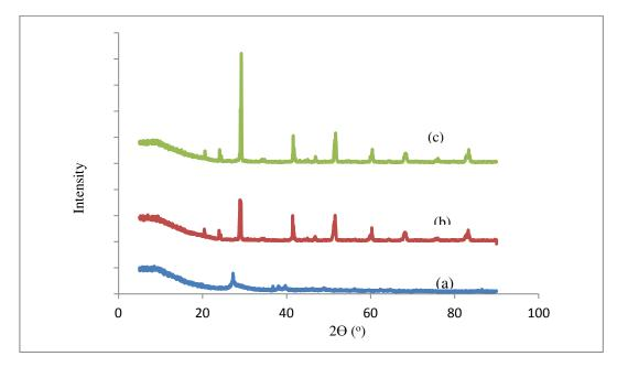
Fig.2. X-ray diffraction pattern of BaBiO<sub>3</sub> at different temperature (a) 300 °C (b) 600 °C and (c) 800 °C
