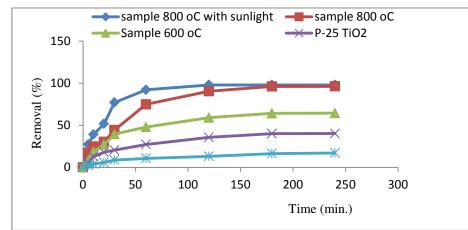
Fig.5. photodegradation curves of diclofenac drug using BaBiO<sub>3</sub> oxide obtained at different calcinations temperature, P-25 TiO<sub>2</sub> and solar light (Drug concentration= 40 ppm; catalyst amount 1g/1000 mL; solution pH=6)
