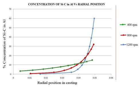
From figure 3 we can see that final position of particle with initial position at 0.005 when process at 800 rpm, gave a result of 21mm radially from centre of casting. When we reduce the rotation speed by 50%, ie to 400 rpm, it reduces the penetration by 62%. When we increase the rpm by 50 %, it increases the penetration to the periphery by 57%. This shows Copyright to IJIRSET www.ijirset.com 14444
