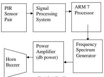
Fig. 4: Basic Flow Diagram
