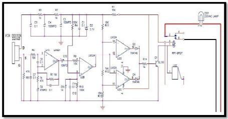
Fig.7: Simulated Circuit Diagram for PIR sensing using NI MULTISIM
