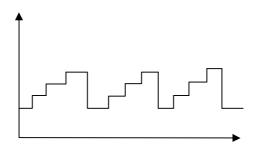
Fig.5. Analog stepped ramp signal
