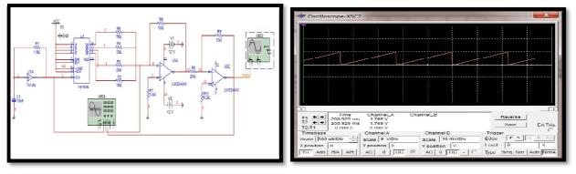
Fig.9: Schematic for Ramp Generator
