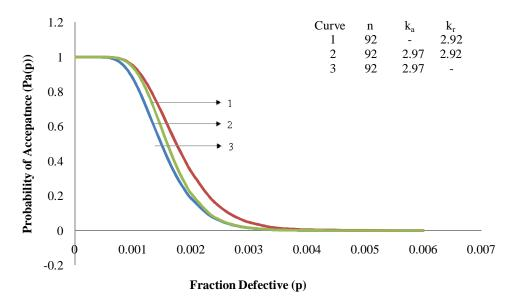
**Figure 1:** The OC curve of MDS-1( $n_{\sigma}$ ;  $k_{\alpha\sigma}$ ,  $k_{r\sigma}$ ) variables sampling plans, curve 1,  $n_{\sigma} = 92$ ,  $k_{r\sigma} = 2.92$ ,  $\alpha = 7$ ,  $\beta = 0$ ; curve 2,  $n_{\sigma} = 92$ ,  $k_{\alpha\sigma} = 2.97$ ,  $k_{r\sigma} = 2.92$ ,  $\alpha = 7$ ,  $\beta = 0$ ; curve 3, n = 92,  $k_{\alpha\sigma} = 2.97$ ,  $\alpha = 7$ ,  $\beta = 0$ ;
