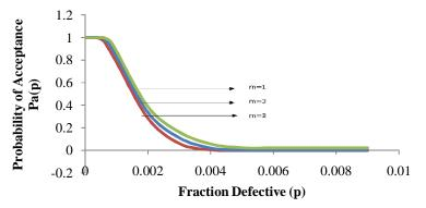
Figure 2: mparison of OC curves with minimum sum of risks for MDS  $n_{\sigma} = 59$ ,  $k_{a\sigma} = 2.90$  and  $k_{r\sigma} = 2.88$  when m=1; $n_{\sigma} = 65$ ,  $k_{a\sigma} = 2.88$  and  $k_{r\sigma} = 2.86$  when m=2; $n_{\sigma} = 71$ ,  $k_{a\sigma} = 2.88$  and  $k_{r\sigma} = 2.86$  when m= 3;
