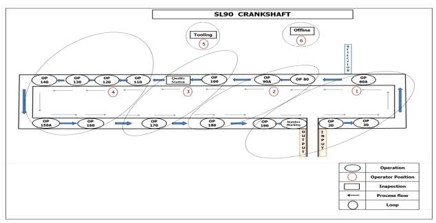
Fig.3 Proposed layout and man-power deployment of SL90 Crankshaft machining line TABLE 1. Operator Engage Time and Their Calculation
