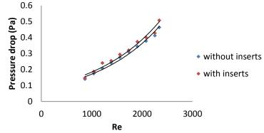
Fig. 7 Variation of pressure drop with Reynolds number for plain tube and with twisted wire brush inserts
