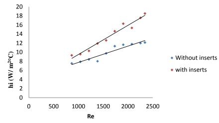
Fig. 5 Variation of inner convective heat transfer coefficient with Reynolds number for plain tube and tube with twisted wire brush inserts
