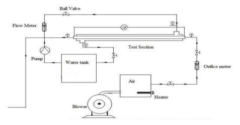
Fig. 1 Block diagram of proposed experimental set-up
