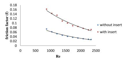
Fig. 6 Variation of friction factor with Reynolds number for plain tube and with twisted wire brush inserts
