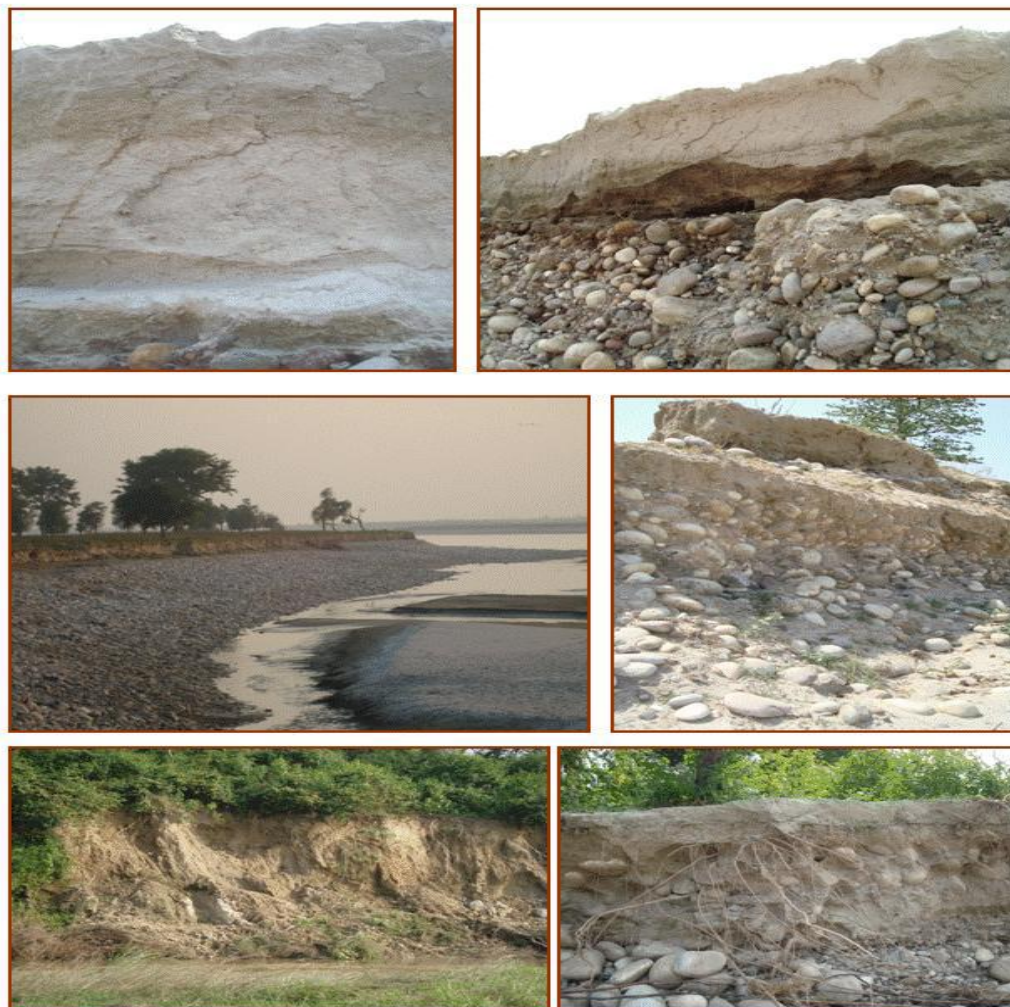
Plate-1: Sediment stratification of River bank of Ganga and other tributaries of the study area
