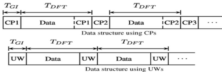
Fig 4 Transmit data structure using cyclic prefix (CPs) & Unique word (UWs)
