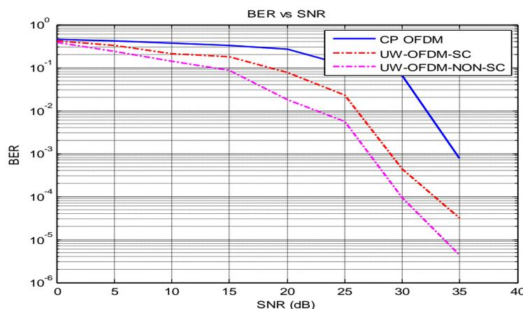
Fig 5 BER comparison between CP-OFDM, UW-OFDM SC & UW-OFDM NONSC
