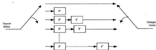
Fig 2 convolution interleave
