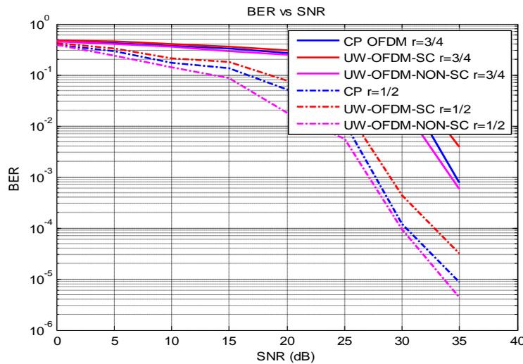
Fig .6 BER comparison between CP-OFDM, UW-OFDM SC & UW-OFDM NONSC with outer coding
