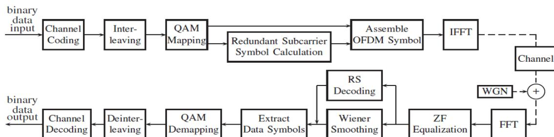
Fig 1: Block diagram of UW OFDM
