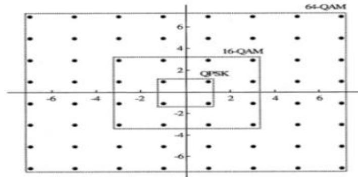
Fig 3 QPSK, 16 QAM & 64 QAM Constellations
