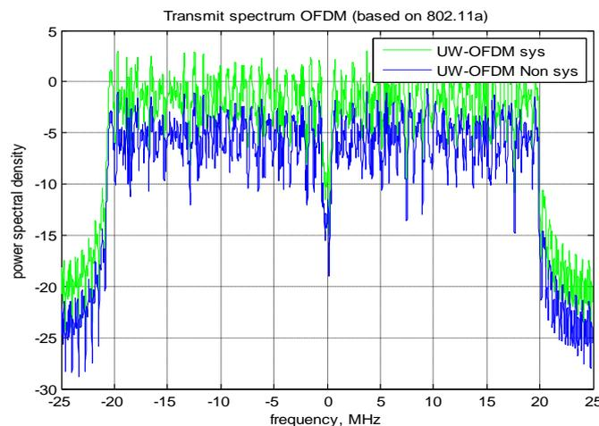
Fig 7 power spectral density comparison UW OFDM systematic and Non Systematic
