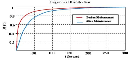
Figure 7: Turbine 2 Maintainability Distribution after Maintenance Procedure Improvement
