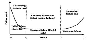
Figure 1: Bath-Tub Curve
