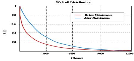
Figure 6: Turbine 2 Reliability Distribution after Maintenance Procedure Improvement
