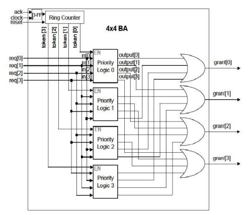
Fig 4.1 Logic Diagram of 4x4 Bus Arbiter
