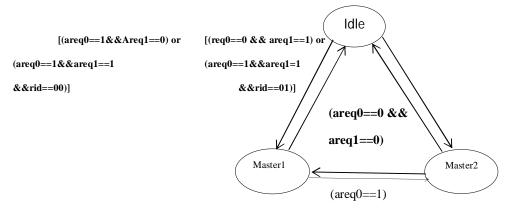
Fig.5.1 State Diagram for Bus Arbiter
