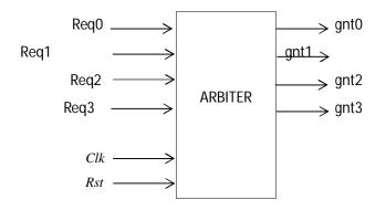
Fig. 3.1Basic block diagram of bus arbiter
