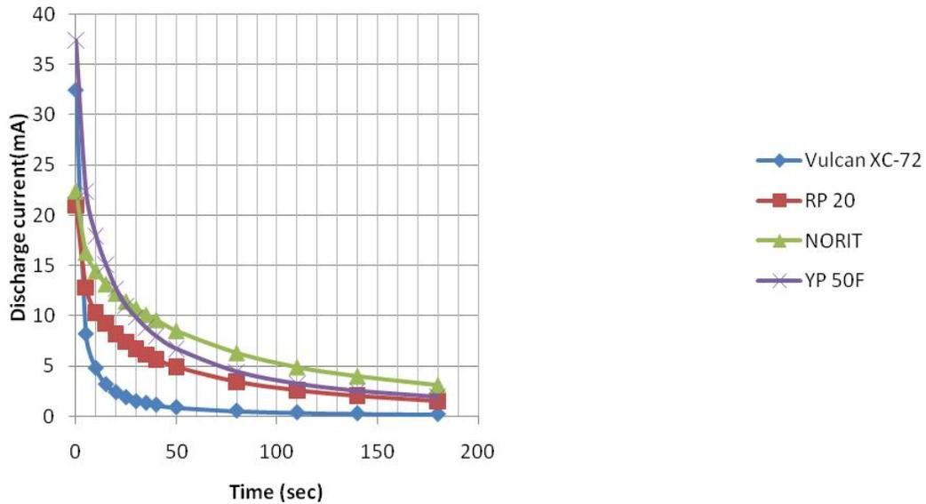
Fig 1 Supercapacitor discharge current characteristics for different carbon materials
