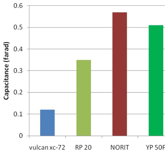
Fig 2 Capacitance of supercapacitors using different carbon materials
