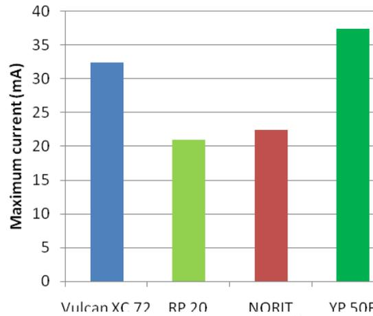
Fig 3 Characteristics of maximum value of current for different types of carbon materials
