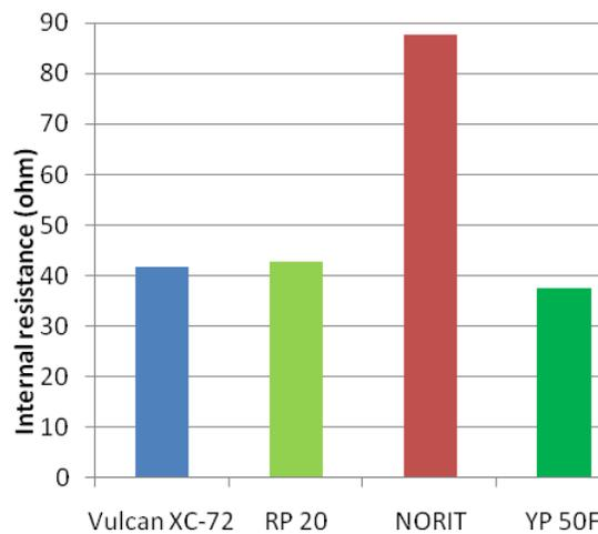
Fig 4: Internal resistance characteristics of supercapacitor for different supercapacitor
