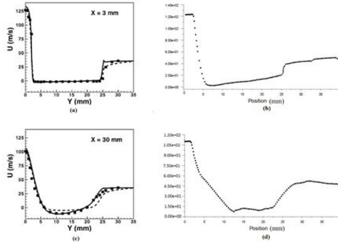
**Figure 6 Experimental results (a) at 3mm & (b) 30mm from BB, Obtained velocity plots (b) at 3mm & (d) at 30mm from BB using RSM**
