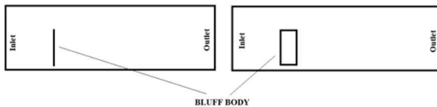
**Figure 9 Geometry of combustion chamber with (a) circular plate and (b) solid cylinder as bluff body**
