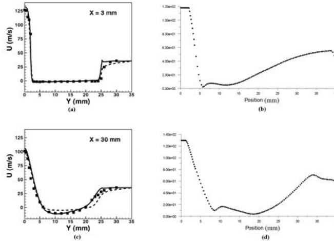
Figure 4 Experimental results (a) at 3mm & (b) 30mm from BB, Obtained velocity plots (b) at 3mm & (d) at 30mm from BB using RNG k-ε model
