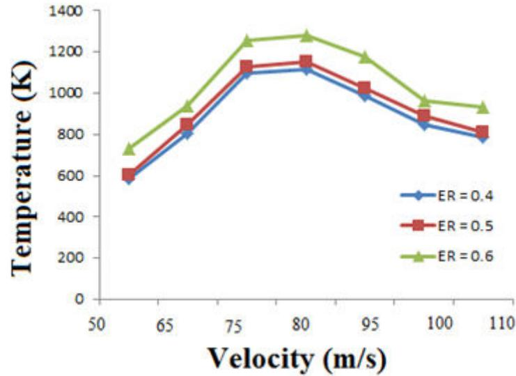
**Figure 8 Values of temperature results obtained with different velocities at an equivalence ratio of 0.4, 0.5, and 0.6**
