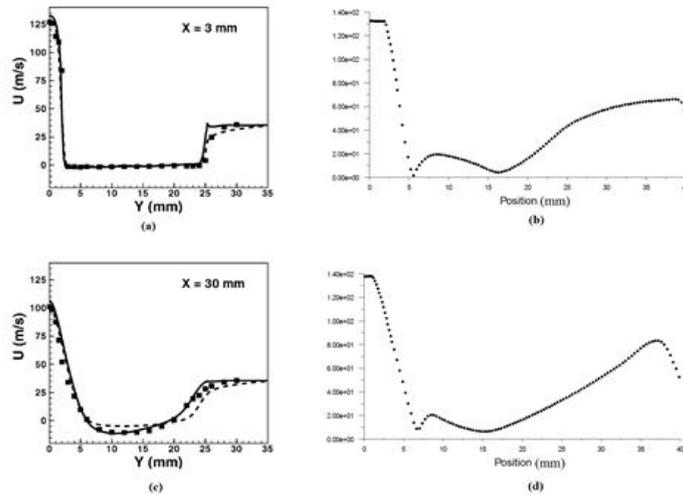
Figure 5 Experimental results (a) at 3mm & (b) 30mm from BB, Obtained velocity plots (b) at 3mm & (d) at 30mm from BB using SST k-ω model
