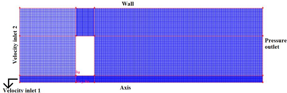
**Figure 2 GAMBIT model for the combustor**
