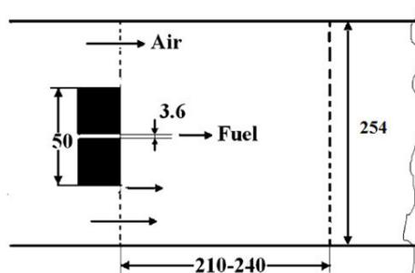
**Figure 1 Schematic of the combustion chamber**
