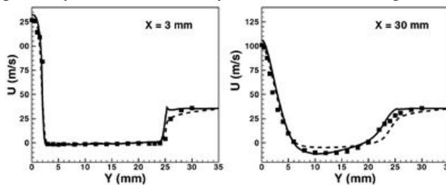
**Figure 3 Experimental velocity values obtained along the radial axis at an axial distance of 3mm and 30mm from the bluff body [12, 13]**
