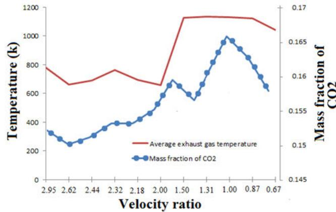
**Figure 7 Values of temperature and CO<sub>2</sub> mass fraction results obtained with different velocity ratios at an equivalence ratio of 0.5**
