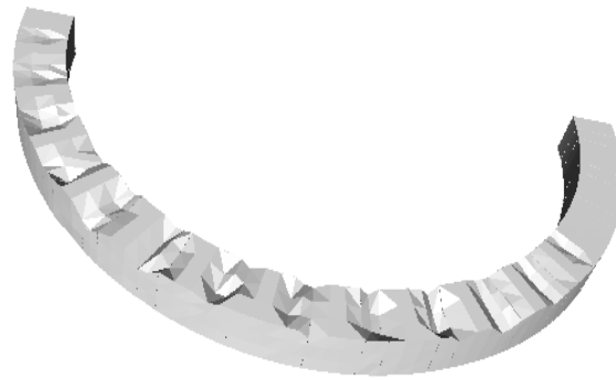
Figure 6. The distribution of contact forces on the ring
