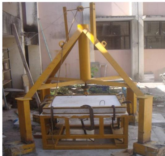
**Fig.1** Experimental set-up for Impact test
