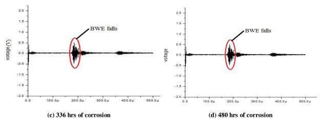
Fig.11: Signatures of 2MHz frequency at location 11
