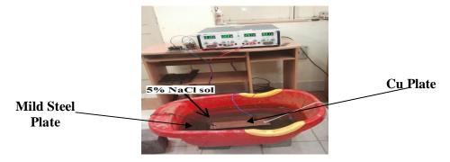
Figure 3: Setup for impressed current corrosion
