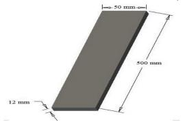
Fig.5: Healthy mild steel plate specimen
