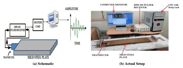
Fig. 5: Ultrasonic Investigations for capturing the wave signatures
