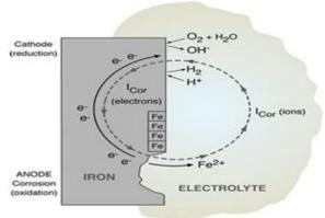
Figure1: Mechanism of Corrosion
