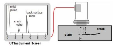
Fig. 4: PE Testing in Plate in Air
