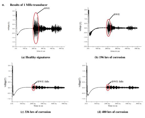
Fig.9: Signatures of 1MHz frequency at location 11
