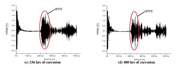
Fig.7: Signatures of 0.5MHz frequency at location 11
