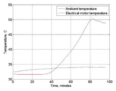
Fig. 6. Time diagram obtained at temperature monitoring of an induction motor.
