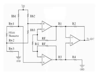
Fig. 4. Diagram of resistive sensors connection
