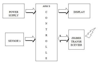
Fig. 3. Block diagram of a temperature measurement end-device.
