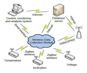
Fig. 1. General structure of the wireless measuring system.
