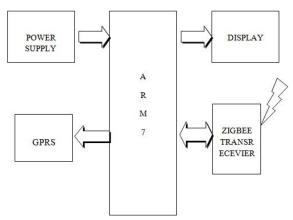
Fig. 2. Block diagram of the data collection module (Coordinator device).
