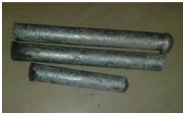
Figure1. Pictorial view casting of sample containing different % SiC by weight
