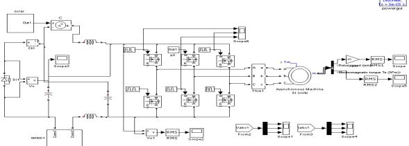
Fig 4a.AC to AC converter for wind generation circuit with induction motor load.
