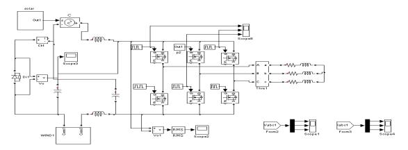
Fig 3a.AC to AC converter for wind generation circuit with RL load.
