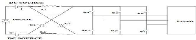
Fig 2. General Structure of EZ-Source Network
