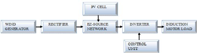
Fig 1.Schematic diagram of wind energy conversion system.
