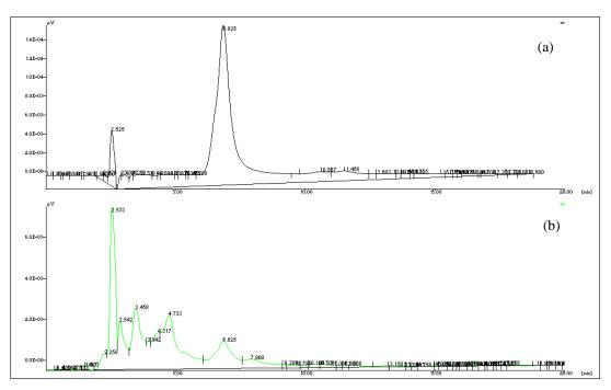
Fig. 6 HPLC chromatogram of (a) purified quercetin fraction collected from silica gel chromatography (a) ethyl acetate extract from cell biomass
