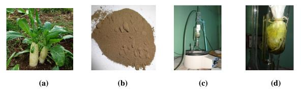
Fig.1: (a) Raphanus sativus (b) Dried leaf powder (c) Soxhlet extractor (d) Quercetin extraction
