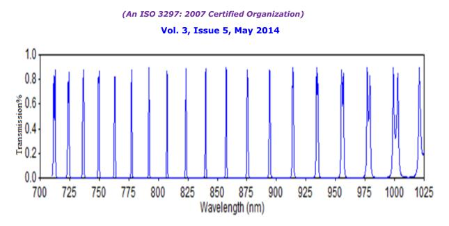
Fig. (1): Transmission vs. wavelength for design multi-cavity sharpness pulses filter with two cavities
