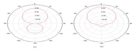
Fig.9 Radiation pattern of: (a). un-optimized ACMPA, (b). optimized ACMPA
