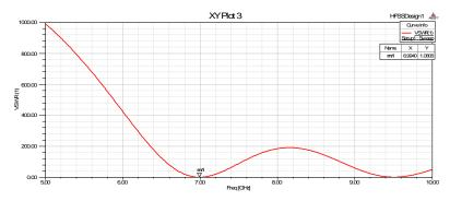
Fig.6 VSWR vs. Freq. plot of the optimized ACMPA
