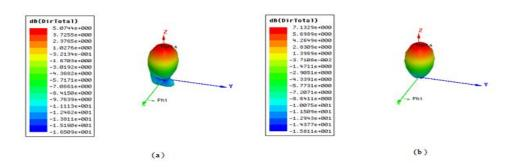
Fig.8 3D polar plot of: (a). un-optimized ACMPA, (b). optimized ACMPA
