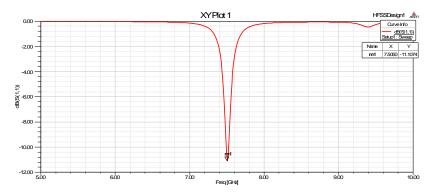
Fig.4 Return loss plot of un-optimized ACMPA
