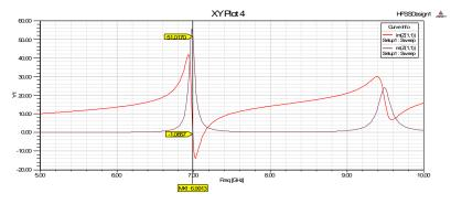
Fig.7 Input impedance variation with frequency
