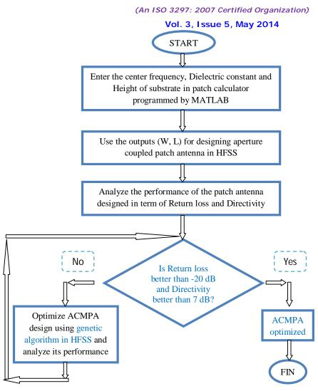
Fig.2 Flow chart showing use of GA in ACMPA design
