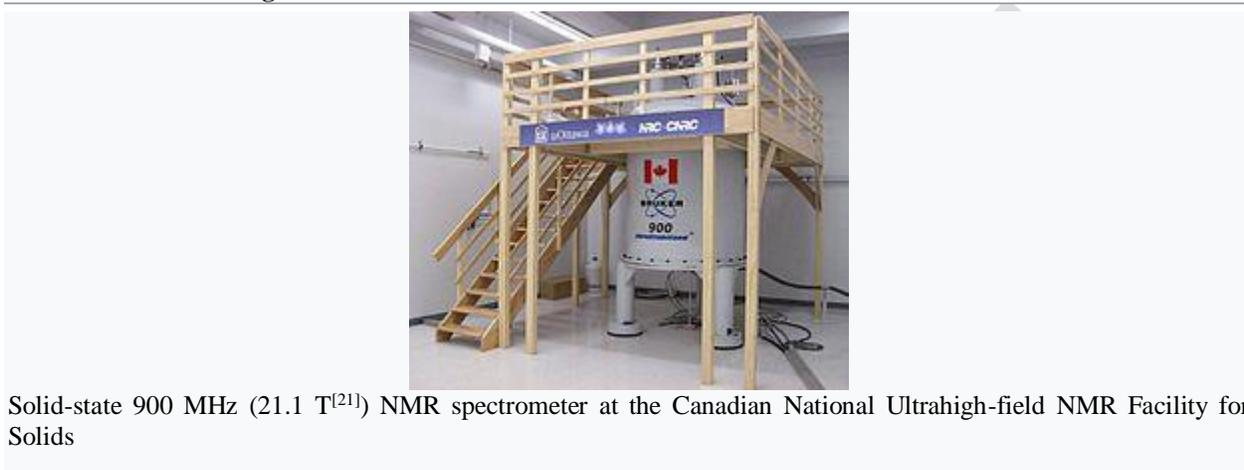
Solid-state 900 MHz (21.1 T<sup>[21]</sup>) NMR spectrometer at the Canadian National Ultrahigh-field NMR Facility for Solids
