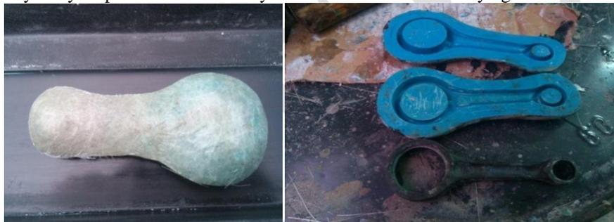
Fig 23: Fiber Glass Mold Preparation
