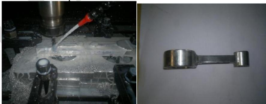
Fig 21: CNC machining of aluminum block
