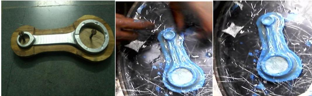
Fig 22: Mold Preparation
