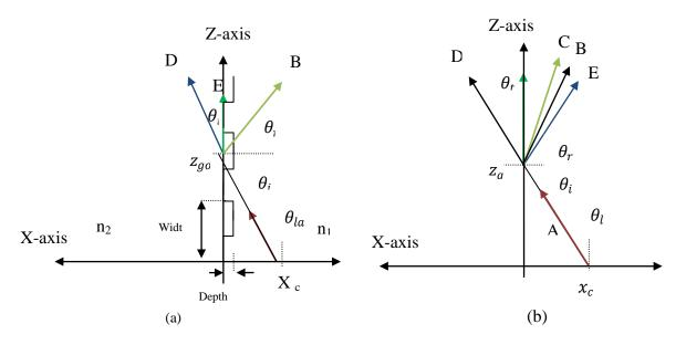
Fig.1: Ray tracing in the simulation (a) with corrugated interface (b) with a planar interface.
