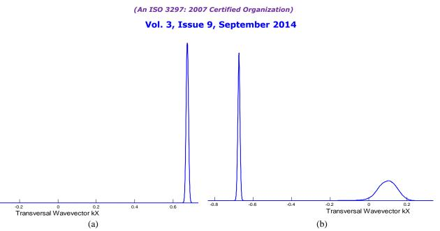
Fig.3: The spectrum for the field (a) input field spectrum, and (b) The output field spectrum in planar interface case.
