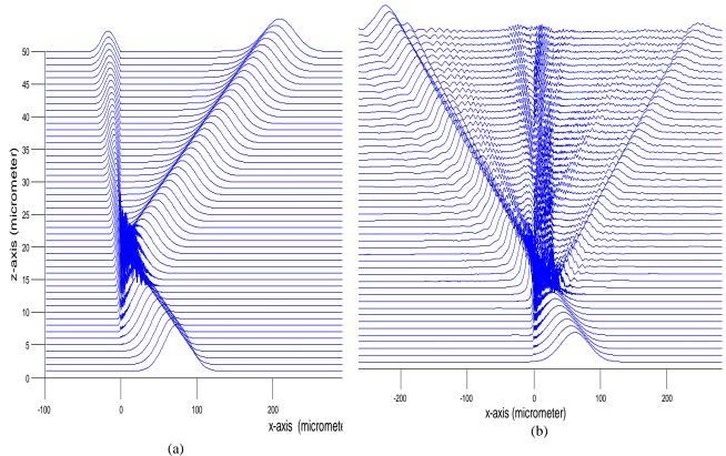
Fig 2: The total field overview at the incident critical angle (a) in planar interface case (b) in corrugated interface case.
