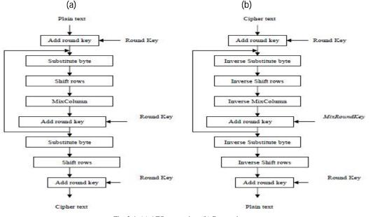
Fig. 2.4. (a) AES encryption, (b) Decryption
