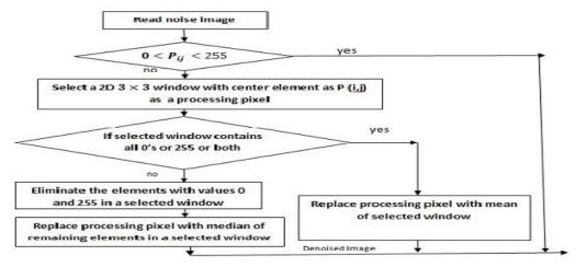
Fig.2.1 Flow chart of MDBUTMF algorithm
