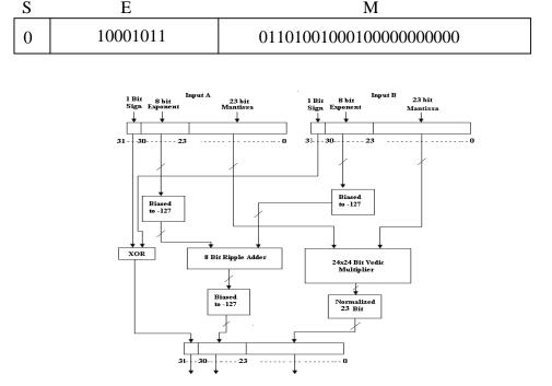
Fig.2: Architecture of Single Precision Floating Point Multiplier.
